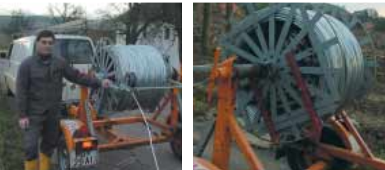
Erwin Grillenberger's idea of using round steel for local network cabling was selected as the idea of the month in March 2003. In the meantime, this winding device is already in use at a number of customer centres.
